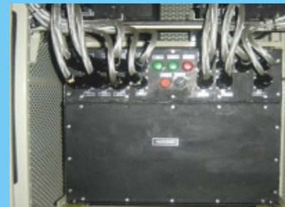
24V-300Amps SMPS in IP65 enclosure
